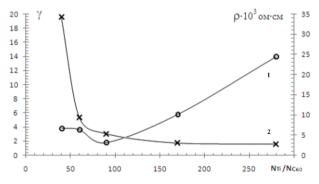
Fig. 1. Change in the coefficient of sensitivity of  $\gamma$  (1) and specific electric resistance  $\rho$  (2) from the fractional ratio  $nTi / nC_{60}$  of the components of titanium-fullerene films.
