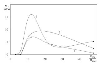
Figure 2. Dependence of the electrical conductivity of  $Cu-C_{60}$  films on different frequencies of alternating current from the calculated number of copper atoms per molecule of  $C_{60}$ : 1 - 1 MHz; 2 - 10 kHz; 3 - 100 Hz.
