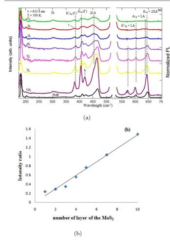
FIG. 2: (a) Resonant Raman spectra of different layers of  $MoS_2$  using 632.8 nm laser line at the 300 k. (b) Calibration curve of the intensity area ratio of the  $MoS_2 E_{2g}^1, A_g^1$  and 2LA Raman modes to that area of the Si substrate. Squares are experimental data, and the line is linear fit.
