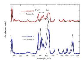
FIG. 4: The Raman spectra before and after annealing in a vacuum  $(300^{\circ}C \text{ for } 40 \text{ min})$ .
