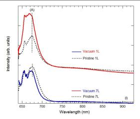
FIG. 5: PL spectra before and after annealing in a vacuum  $(300^{\circ}C \text{ for } 40 \text{ min}).$
