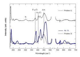
FIG. 6: The Raman spectra before and after annealing in the air  $(300^{\circ}C \text{ for } 40 \text{ min})$ .
