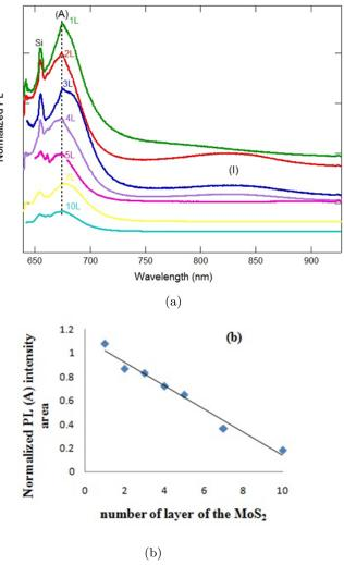
FIG. 3: (a) Normalized PL spectra of different layers of  $MoS_2$ . (b) Calibration curve of the normalized PL intensity area I(A). Squares are experimental data, and the line is linear fit.
