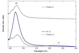
FIG. 7: PL spectra before and after annealing in the air  $(300^0 C \text{ for } 40 \text{ min}).$
